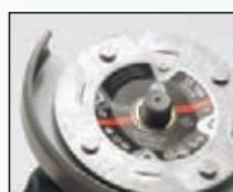
CMT backing plate on angle grinder.
