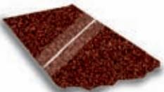
**NO.4** "Butt splice", in which belt ends are butted together and joined by high strength tape on underside of joint. Allows belt to run in either direction for greater belt life and convenience. Smooth running. Most popular splice, suitable for a wide variety of applications and belt sizes. Strongest of the non-specialty joints.
