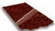
**NO.2** Belt ends are overlapped with partial grain removed off top of splice (partial top-skived). Smooth running over platens or hard contact wheels for cloth belts 80 grit or finer. Seen mainly on edge sanders where bull nose or dead head sanding is being done.
