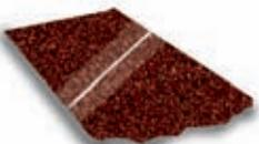
**"T" Joints** A top skived #4 butt joint used on cloth belts 150 and finer for platen sanding operations on wide belt sanders or in grits 80 and finer on other belt operations where chatter is a problem when using a #4. Not for use on paper belts. Cloth only.
