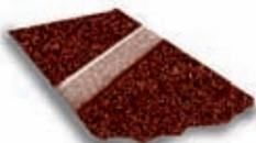
**NO.6** Belt ends are overlapped with a complete grain removal off top of splice (fully top-skived) and cut at a 45 degree angle minimizing the amount of time the joint is in contact with the workpiece. Used where a high degree of conformability in the joint area is required, such as in mold sanding. For cloth belts only!
