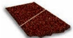
**NO.1** Belt ends are overlapped with no grain removed off top of splice. Offers maximum protection against wear in the lap joints. For soft contact wheels, slack of belt operations and paper belts 150 and finer used in wide belt or lever stroke sanding. Standard joint for pump sleeves.
