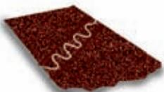
**NO.3** Similar to Type 4 joint except the two belt ends are cut in an interlocking configuration, or zig-zag. Can be run in either direction. Available in grit size 80 or finer only. Designed specifically for glass grinding operations. Not for use on any paper belts.
