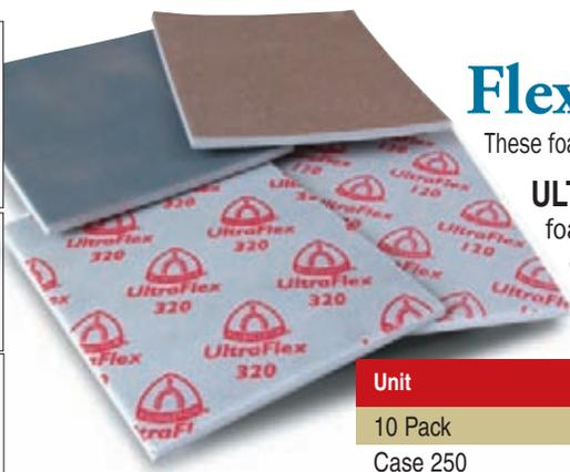
**ULTRAFLEX SANDING PADS** The UltraFlex Sanding Pads are the premium foam pads on the market. These incorporate a dense foam structure and a full, even coating of either aluminum oxide or silicon carbide grains. This makes for an extremely long-lasting pad that is very flexible for finish-sanding of contoured parts and profiles. The pad measures 4 1/2" wide and 5 1/2" long.
