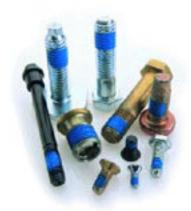
The NYLOK® BLUE® PATCH self-locking element is permanently spray bonded onto the threads of a fastener. When mating threads are engaged, the tough, resilient blue nylon patch element is compressed and a counterforce is created to establish a much stronger metal-to-metal contact and positive resistance to vibration and loosening.
