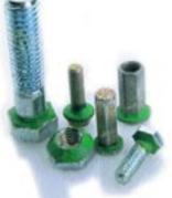
Green-colored NYSEAL creates a gasket-type seal, preventing leakage of fluids and gases under pressures up to 500 psi. The coating is permanently fused on the bearing surface of the fastener. As the screw is seated to its final position against the mating part, the NYSEAL element compresses slightly and fills the void under the bearing surface of the head and countersink/counterbore.
