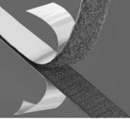
When the two sides of a 3M<sup>™</sup> Scotchmate<sup>™</sup> Hook and Loop Fastener are pressed together, hundreds of tiny, stiff hooks mesh with a surface of pliable loops. Simply press together to fasten and pull apart to open. You'll be able to do it thousands of times during the life
