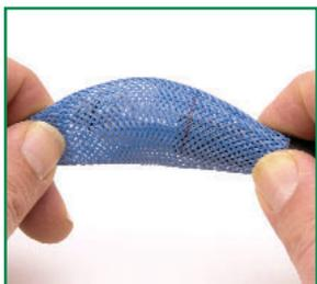
Slip the additional length of sleeving over the end of your application so that the mark is at the spot on the installation where you want the sleeving to end. On this low pressure air hose, it's just below the connector.
