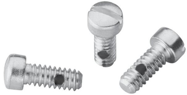
Tek-Lok® self-locking threaded fasteners obtain locking action from an engineered plastic pellet compressed into a hole drilled in the threaded region of the fastener, to a depth slightly below the root of the thread. Pellet size and location are standard but can be altered to meet special requirements.
