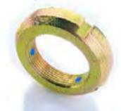
The NYLOK<sup>®</sup> BLUE<sup>®</sup> PELLET and TORQ-STRIP<sup>®</sup> self-locking elements are permanently embedded in the threads of a fastener. When mating threads are engaged, the tough, resilient Blue<sup>®</sup> nylon element is compressed and a counterforce is created to establish a much stronger contact and positive resistance to vibration and loosening.
