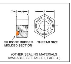
JAM-NUT MATERIAL: Nickel-plated brass can also be made of carbon steel, stainless-steel, aluminum, etc.
