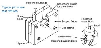
\*Orientation during testing is specification dependent
