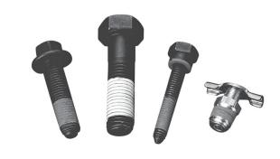
Vibra Seal® Preapplied Thread Sealant is a tough, non-hardening sealant engineered to be preapplied to parts. Vibra-Seal is designed to provide an instant seal on tapered pipe threads against most fluids, fuels and lubricants but can also be used on straight threads. Vibra-Seal performs to the demanding requirements of the automotive, truck and agricultural equipment manufacturers. It provides lubricity superior to Teflon®—at a lowercost!
